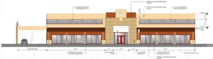
A1 BLDG C - ELEVATION SOUTH 1/8" = 1'-0"
